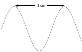
If this wave were an electromagnetic wave, and not a drawing on a page, the wavelength is 5 cm (or 0.05 meter). Using the formula above, that gives us a frequency of 300,000,000/0.05, or 6 billion Hertz. That's around the frequency used by many radars.
