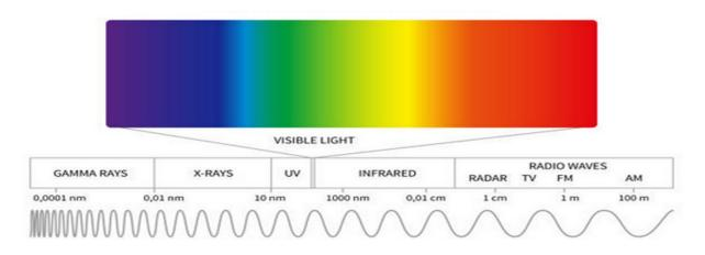
Here's a view of the electromagnetic spectrum. Light occupies just a sliver:
